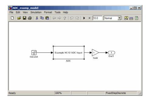
ADC\_examp illustrates a number of techniques for parameterizing a driver by letting the user enter hardware-related variables. Dialog Box for ADC\_examp Driver Block on page 10-20 shows the dialog box that ADC\_examp presents to the user. To launch the dialog box, right-click the ADC S-Function block in the model and select **Mask Parameters**. Parameter values are shown at their default values.
