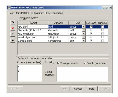
The preceding figure shows how the parameter section of the mask is defined for the ADC\_examp driver. In the ADC\_examp driver, block parameters are declared nontunable in the block mask. If you do not do this, you can declare parameters nontunable by using the ssSetParameterTunable macro in the mdlInitializeSizes routine. Nontunable S-function parameters become constants in the generated code, improving performance.
