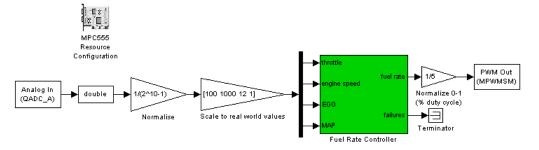
The preceding figure shows a separate version of the model that is specifically targeted for code generation for the Freescale<sup>TM</sup> MPC555 processor. This model contains the same controller block, but the controller is connected
