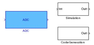
Rather than using the conventional manual selection method (the Configurable Subsystem's **Block Choice** context menu), the ADC Configurable Subsystem block has mask initialization code that makes the selection automatically, depending on whether the model is in simulation or code generation mode. The mask initialization code is listed below.
