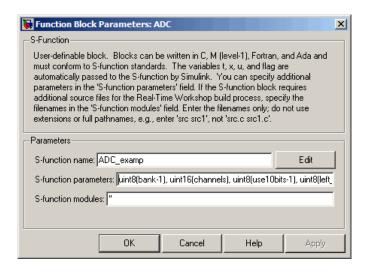
The block parameters underlying the mask, as shown in the preceding figure, provide a binding to the C-MEX S-function for use in simulation, and a list of parameter variables corresponding to the **S-function parameters** field. Note that:
